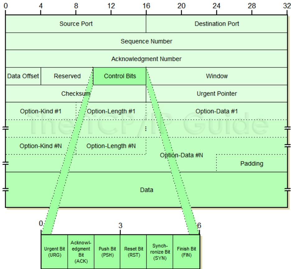
The source port and destination ports identify the endpoints of the transmission. Every port combined with its IP Address form a unique endpoint.
