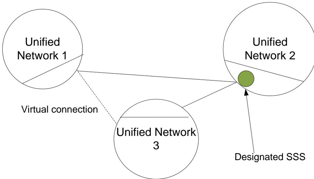
It can be observed in the diagram that Networks 1 and 3 connect through the Designates SSS installed in Network 2 that also share the same SSS with the rest.
